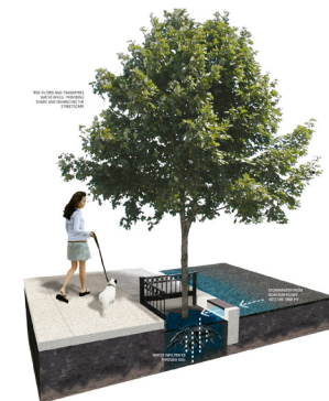
Figure 30: Three-Dimensional View of a Stormwater Tree from the City of Philadelphia (2014).
