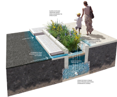
Figure 27: Three-Dimensional View of a Stormwater Planter from the City of Philadelphia (2014).
